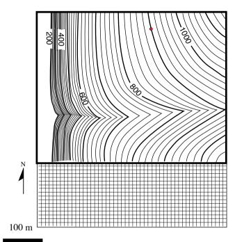
e/ Construct the trace of the vertical plane N150-90 containing the point P.
