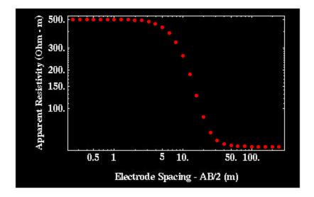
In the example shown above, we acquired the data such that there are 9 soundings for every decade (power of 10) in distance beginning at 0.25 meters. Thus, soundings with current electrode separations, *AB/2*, of 0.25, 0.5, 0.75, 1.0, 1.25, 1.5, 1.75, 2.0, 2.25, 5.0, 7.5, 10.0, 12.5, 15.0, 17.5, 20.0, 22.5, 50.0, 75.0, 100.0, 125.0, 150.0, 175.0, 200.0, and 250.0 meters were taken.
