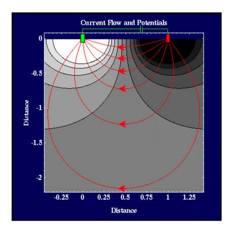
Instead of the current flowing radially out from the current electrodes, it now flows along curved paths connecting the two current electrodes. Six current paths are shown (red lines). Between the surface of the earth and any current path we can compute the total proportion of current encompassed. The table below shows this proportion for the six paths shown above. Current paths are labeled 1 through 6 starting with the top-most path and proceeding to the bottom-most path.
