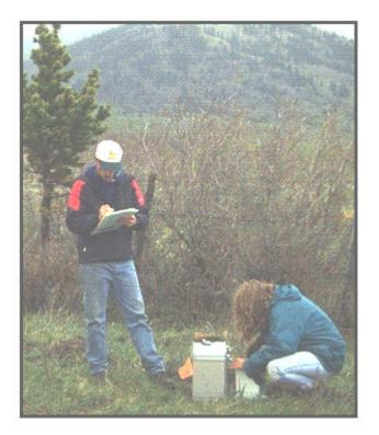
• In conducting active geophysical surveys, on the other hand, a signal is injected into the earth and we then measure how the earth responds to this signal. These signals could take a variety of forms such as displacement, an electrical current, or an active radiometric source. The final two survey methods considered in this short course, DC resistivity and seismic refraction, are examples of active geophysical experiments.
