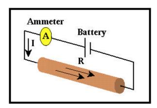
In principle, it is relatively simple to measure the resistance of a strand of wire. Connect a battery to a wire of known voltage and then measure the current flowing through the wire. The voltage divided by the current yields the resistance of the wire. In essence, this is how your multimeter measures resistance. In making this measurement, however, we must ask two crucial questions.
