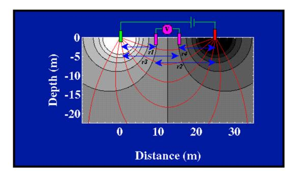
The <u>potential</u> computed along the surface of the earth is shown in the graph below. The voltage we would observe with our voltmeter is the <u>difference in potential</u> at the two voltage electrodes,  $\Delta V$ . The horizontal positions of the four electrodes, two current (red and green) and two potential (purple), are indicated along the top of the figure.
