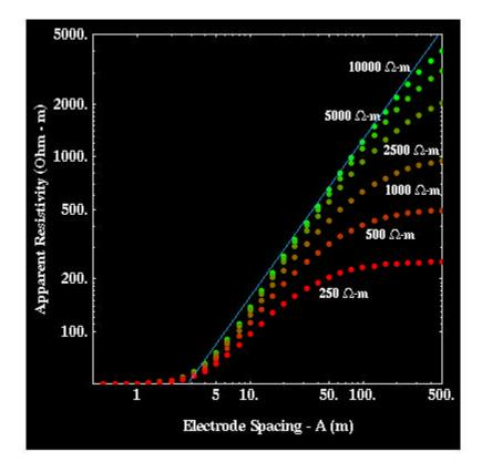
In this example, notice that over the electrode spacing range considered (0.5 to 500 meters), the apparent resistivity curve never approaches the resistivity of the halfspace for halfspace resistivities above 2500 ohm-m. Instead, the apparent resistivity curve approaches a straight line having a slope of 45 degrees
