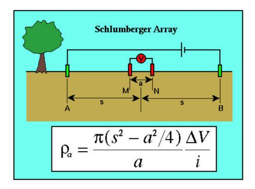
The current electrodes are at equal distances from the center of the sounding, s. The potential electrodes are also at equal distances from the center of the sounding, but this distance, a/2, is much less than the distance s. Most of the interpretational software available assumes that the potential electrode spacing is negligible compared to the current electrode spacing. In practice, this is usually interpreted to mean that a must be less than 2s/5.
