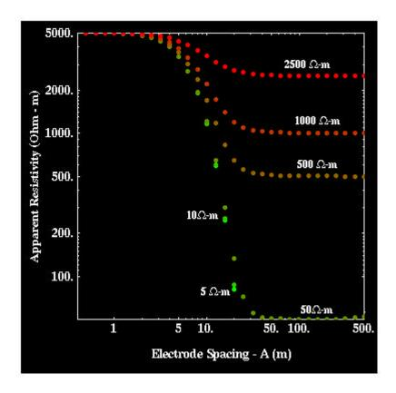
In this particular case, the apparent resistivity curves behave exactly as we would expect them to, given what we have seen in our previous examples. All of the curves asymptotically approach the resistivity of the layer, 5000 ohm-m, at small electrode spacings. As electrode spacing increases, the apparent resistivity curves asymptotically approach the true resistivity of the halfspace (this is true even for the 10
