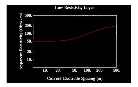
Because current would prefer to flow within the first layer, notice that the apparent resistivity approaches the resistivity of the halfspace more slowly (i.e., with greater electrode spacings) than was found in the <u>previous</u> case.
