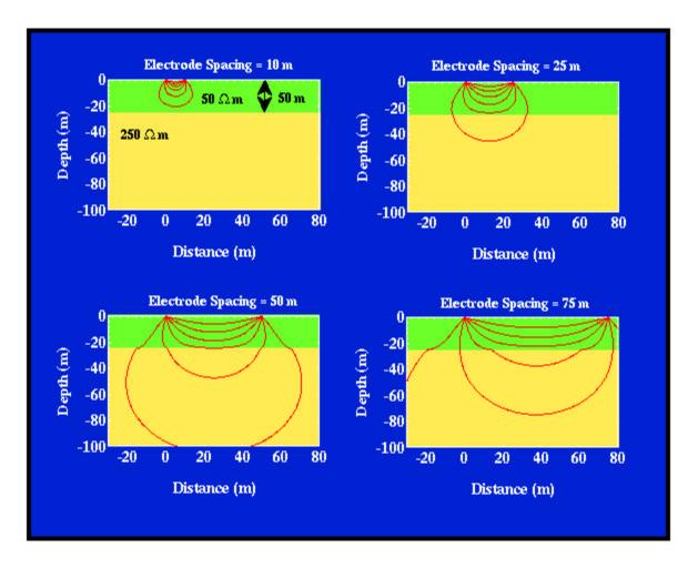
Initially with the current electrodes closely spaced, most of the current is confined to the upper layer along paths that are very close to those that they would have assumed if the model were homogeneous. The computed apparent resistivity is very close to the resistivity of the upper layer, 50 ohm-m.
