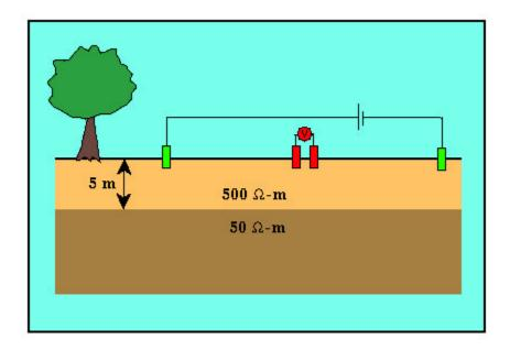
Let's do our Schlumberger sounding by varying current electrode spacing, <u>AB/2</u>, from 1 to 250 meters at 1 meter increments. Shown below is a plot of the resulting apparent resistivity versus electrode spacing.
