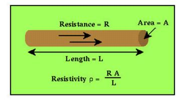
In the case of a wire, resistivity is defined as the resistance in the wire, times the cross-sectional area of the wire, divided by the length of the wire. The units associated with resistivity are thus, ohm - m (ohm - meters).
