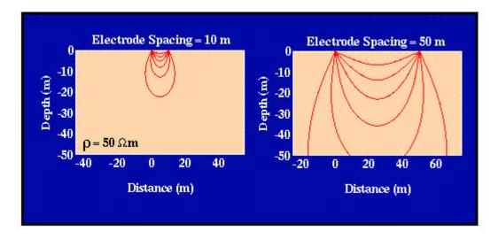
What this implies is that by increasing the electrode spacing, more of the injected current will flow to greater depths, as indicated in the figure above. Because the total resistance in the electrical path increases as electrode spacing is increased, to get current to flow over these longer paths requires a larger generator of electrical current. Thus, the maximum distance that current electrodes can be separated by is in part dictated by the size of the generator used to produce the current.
