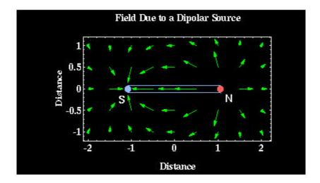
The force associated with this fundamental element of magnetism, the magnetic dipole, now looks more complicated than the simple force associated with gravity. Notice how the arrows describing the magnetic force appear to come out of the monopole labeled *N* and into the monopole labeled *S*.
