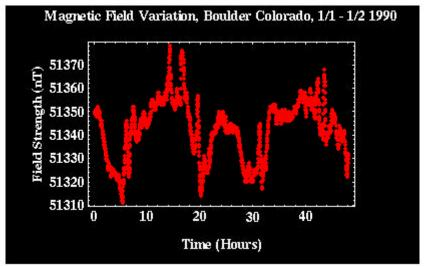
These variations are believed to be caused by electric currents induced in the Earth from an external source. In this case, the external source is believed to be electric currents in the upper atmosphere, or the ionosphere. These electric currents in the ionosphere are in turn driven by solar activity.
