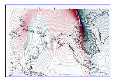
If the Earth's field were simply dipolar with the axis of the dipole oriented along the Earth's rotational axis, all declinations would be 0 degrees (the field would always point toward the north). As can be seen, the observed declinations are quite complex.
