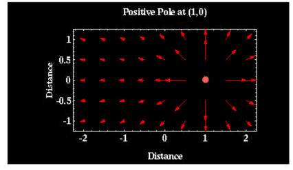
\*For plotting purposes, the arrow lengths shown in the figures above decay proportional to one over the distance between the two poles rather than proportional to one over the square of the distance between the two poles. If the true distance relationship were used, the lengths of the arrows would decrease so rapidly with distance that it would be difficult to visualize the distance-force relationship being described.
