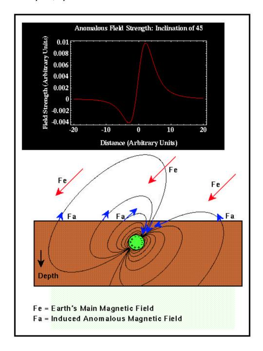
As in the previous examples, the Earth's main magnetic field induces an anomalous field in surrounding the sphere. The anomalous field is now oriented at some angle, in this case 45 degrees, from the horizontal. By looking at the direction of the anomalous field, Fa, in comparison with the Earth's main field, Fe, you can see that there will be a small negative anomaly far to the south of the sphere, a large
