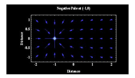
As described by Coulomb's equation, the size of the arrows should decrease as one over the square of the distance between the two magnetic poles\* and the direction of the force acting on p2 is always in the direction toward p1 (the force is attractive)\*\*.
