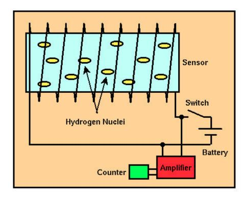
The sensor component of the proton precession magnetometer is a cylindrical container filled with a liquid rich in hydrogen atoms surrounded by a coil. Commonly used liquids include water, kerosene, and alcohol. The sensor is connected by a cable to a small unit in which is housed a power supply, an electronic switch, an amplifier, and a frequency counter.
