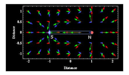
If we add these forces together using *vector addition*, we get the green arrows. These green arrows now indicate the force associated with a magnetic dipole consisting of a negative monopole at x=-1, labeled S, and a positive monopole at x=1, labeled S. Shown below are the force arrows for this same magnetic dipole without the red and purple arrows indicating the monopole forces.
