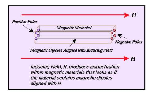
The strength of the magnetic field induced by the magnetic material due to the inducing field is called the *intensity of magnetization*, *I*.
