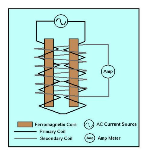
The fluxgate magnetometer is based on what is referred to as the *magnetic saturation circuit*. Two parallel bars of a <u>ferromagnetic</u> material are placed closely together. The <u>susceptibility</u> of the two bars is large enough so that even the Earth's relatively weak magnetic field can produce magnetic saturation\* in the bars.
