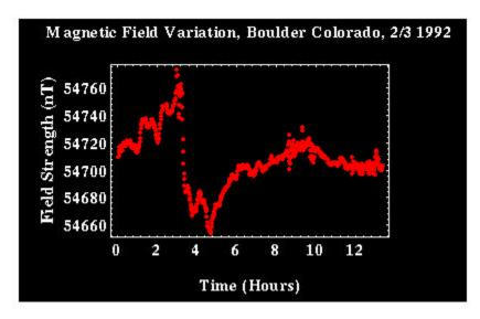
location during such a transient event. Although the magnetic storm associated with this event is not particularly long-lived, notice that the size of the magnetic field during this event varies by almost 100 nT in a time period shorter than 10 minutes!!
