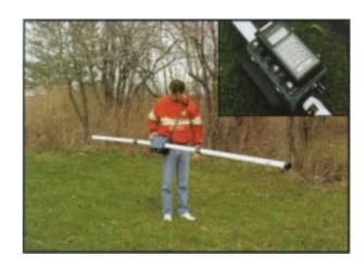
magnetic inductive technique that makes the measurements without electrodes or ground contact. With this inductive method, surveys can be carried out under most geological conditions including those of high surface resistivity such as sand, gravel and asphalt.
